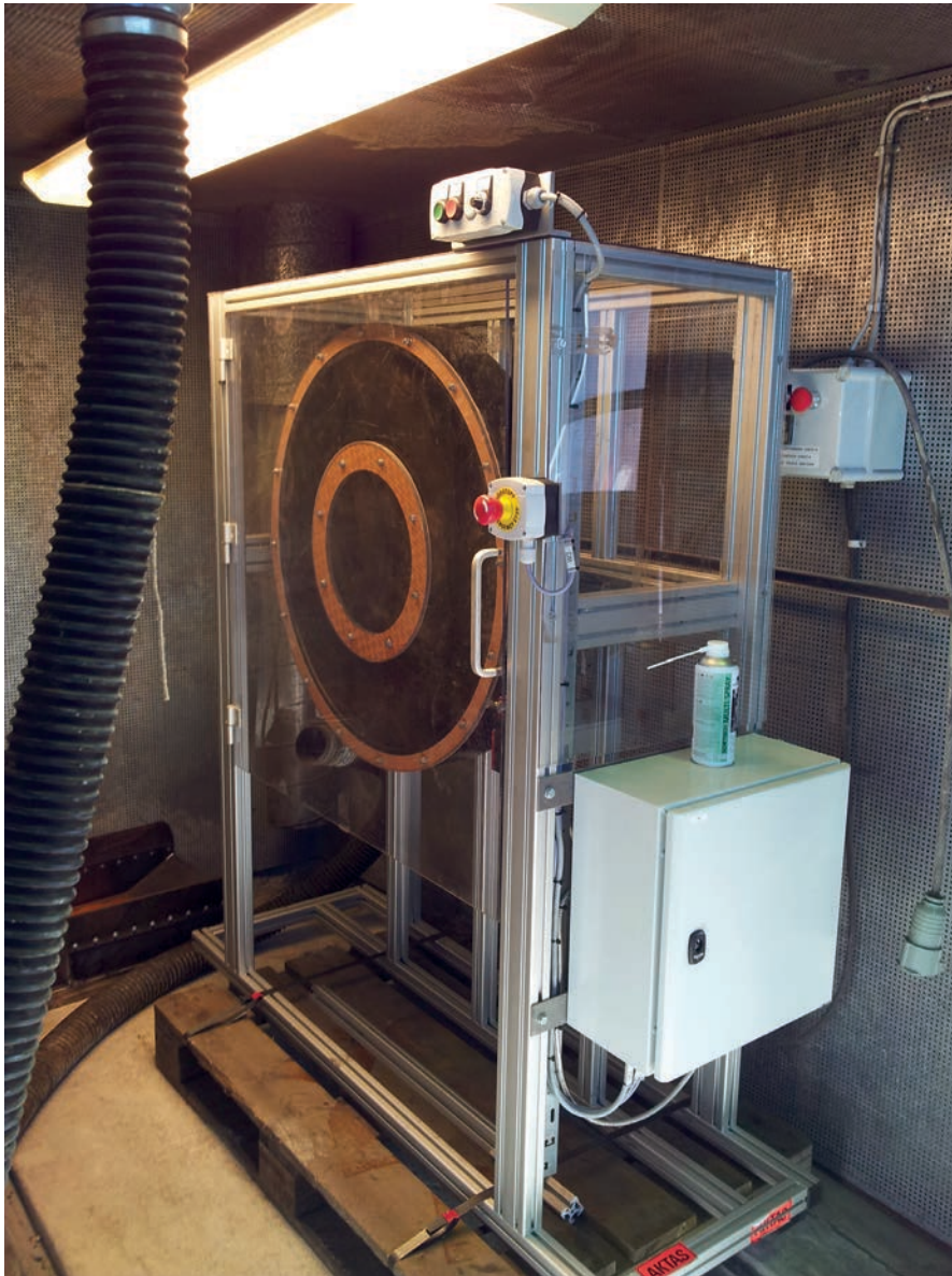
SSAB's Drum Wear Test consists of an \text{R}800 \times 100 \text{mm} steel drum, where up to 34 samples are placed in a holder, assembled along the inside of the drum and tested under the same conditions.
